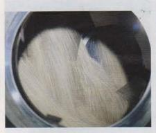
Rotary batch mixing action - cut, turn, tumble, fold - achieves uniform blends in one to three minutes per batch.
