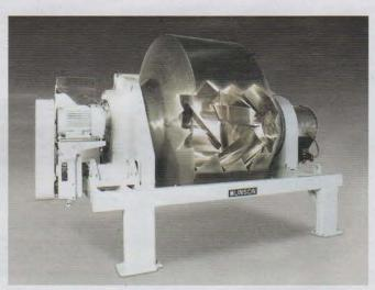
Staggered mixing flights create a four-way mixing action that uniformly distributes ingredients with little or no degradation or frictional heat
